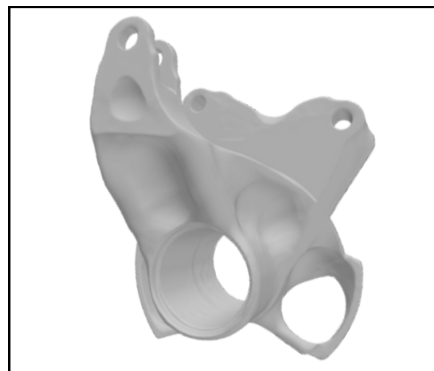
Optimized bracket for 5-axis CNC Machining
